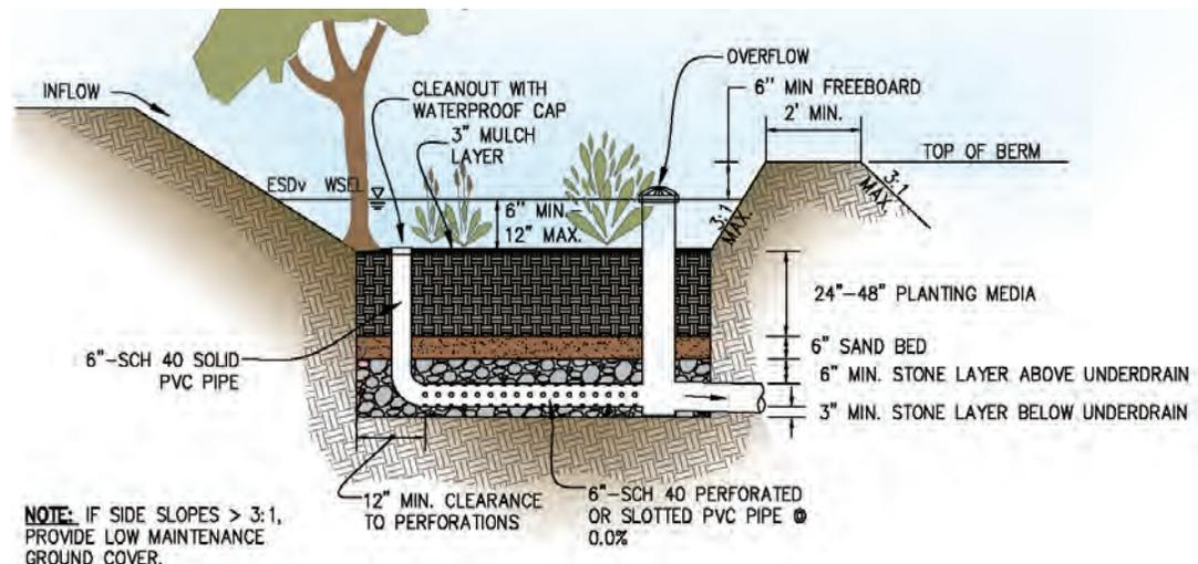
**Figure 3: Illustration of Bio-swale**
