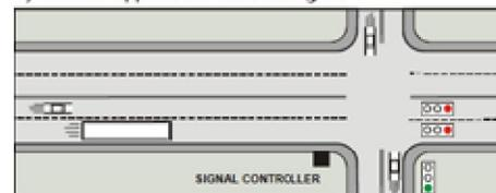
2) The signal controller detects the bus; it terminates side street green phase early
