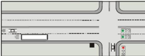
2) The signal controller detects the bus; it extends the current green phase
